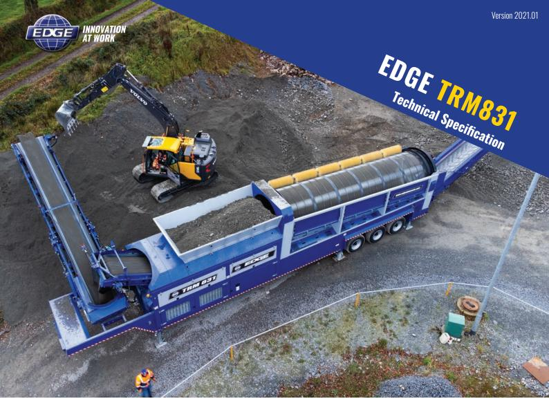
One of the largest mobile trommels available; the EDGE TRM831 offers high production rates with extensive stockpiling capacities thanks to its end discharge conveyor design and remote 180° radial fines conveyor.
