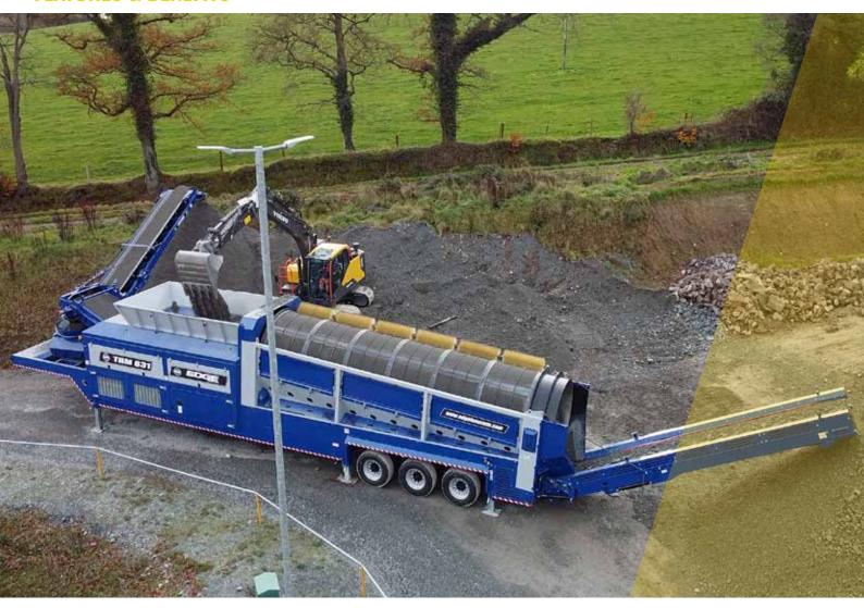
One of the largest mobile trommels available; the EDGE TRM831 offers high production rates with extensive stockpiling capacities thanks to its end discharge conveyor design and remote 180° radial fines conveyor.
