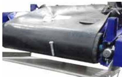
Magnetic Head Drum -fit to either discharge conveyors
