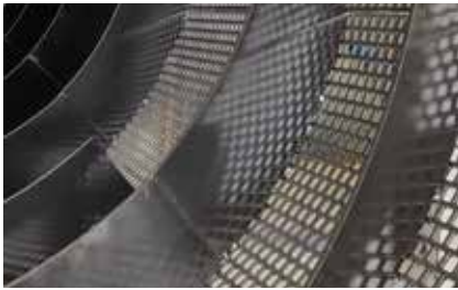
Spiral Drum - ideal for extending screening time of feed material
