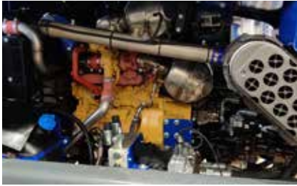
Tier 4 Final / STAGE V - CAT3.6 100Kw (134HP)
