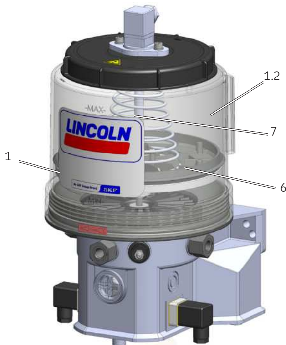
Overview, functional description of pumps with follower plate Fig. 3
