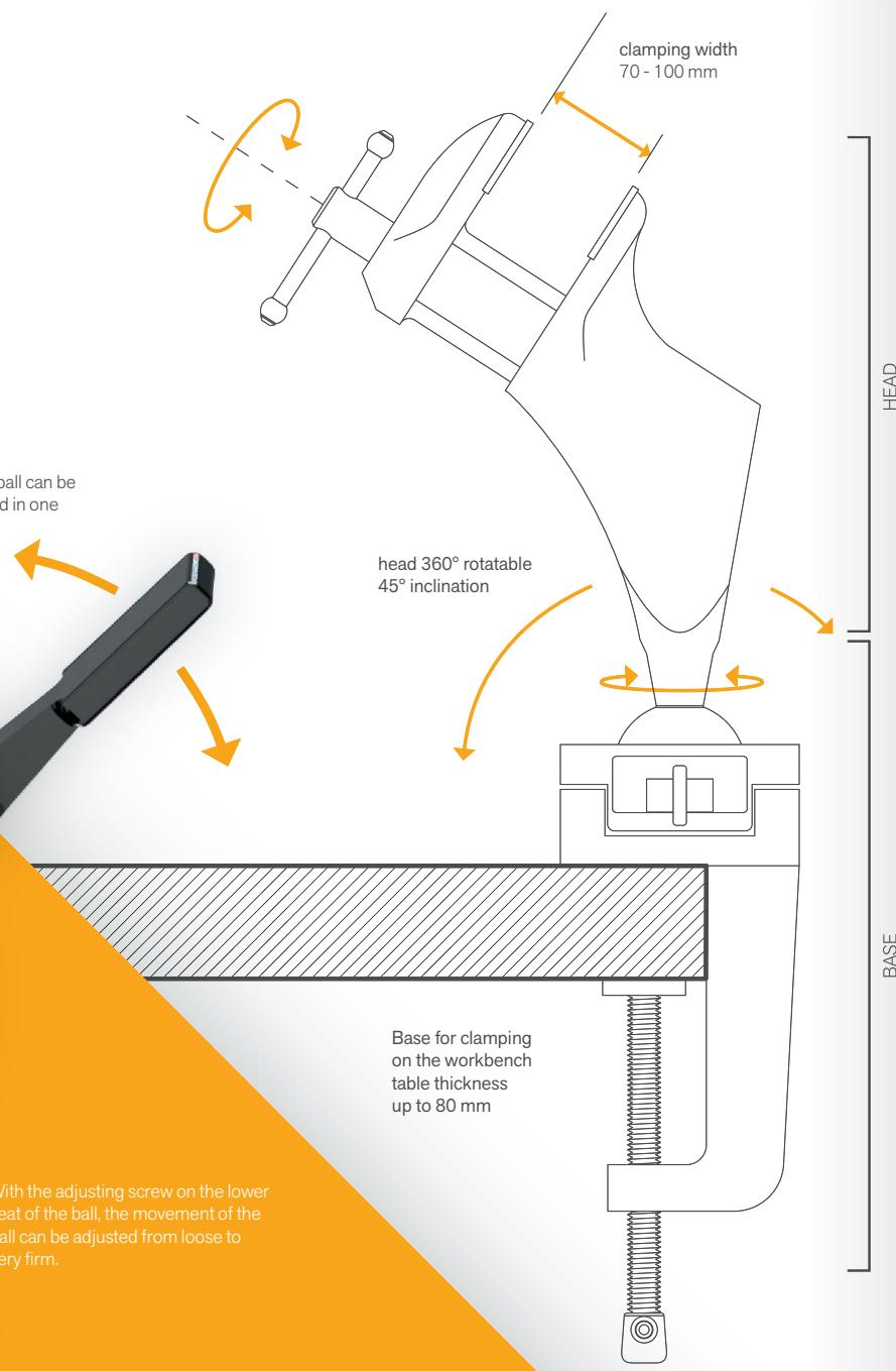
With the adjusting screw on the lower seat of the ball, the movement of the ball can be adjusted from loose to very firm.
