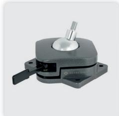
The holder can be screwed to the workbench through 4 through holes (space dimensions 152 x 151 mm), or it can be fixed to steel surfaces with 4 magnets. The 4 high-performance magnets with protective caps have a holding force of 32 kg horizontally and 15 kg vertically (magnets without caps). The magnets are firmly connected to the housing with screws. A drilling drawing can be downloaded from the website.
