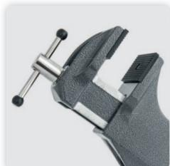
With 4 high-performance magnets (including protective caps) for fixing to steel surfaces. Holding force 32 kg horizontal, 15 kg vertical (magnets without caps). The magnets are firmly connected to the base by screws. A small lever pressure is sufficient and the clamped workpiece can be fixed steplessly and in any practical working position.
