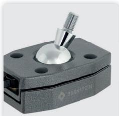
This slim holder is the lightweight among the BERNSTEIN holders. At 110 x 72 mm, it can be screwed onto any tabletop with 4 through holes (Ø 6.5 mm) to save space, or fixed to steel surfaces with 4 magnets. A drilling drawing can be downloaded from the website. The 4 heavy-duty magnets with protective caps have a holding force of 32 kg horizontally and 15 kg vertically (magnets without caps). The magnets are firmly connected to the base by screws.
