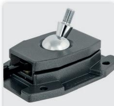
Suitable for all workbenches and tables. Place dimensions 150 x 106 mm. The holder can be screwed on with four through holes (Ø 9 mm). A drilling drawing can be downloaded from the website. A small lever pressure is sufficient to fix the ball steplessly and in any practical working position.
