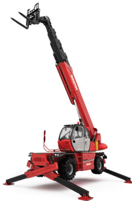
Rotation on lowered stabilizers with 1500 kg jib
