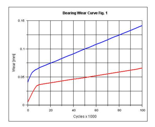
It will be noted that a wear-in period takes place during the first few thousand cycles. During this period some PTFE is transferred to the mating surface. In addition, the fibres are generally reoriented, the high spots of the weave are flattened and adjacent fibres tend to blend together. After the break-in period, the bearing surface will become smooth and shiny.
