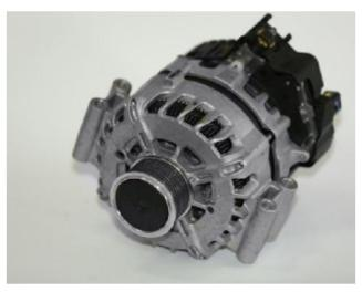
The system is based on a reversible electric mo-tor that serves the functions of both starter and alternator. The reversible alternator can easily be mounted in the place of the classical one. It permits a very gentle start-up. In comparison with the conventional starter, there is no cou-pling process, so no additional sounds connect-ed with this operation are emitted.
