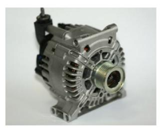
The moment the engine is put in motion, the alternating voltage stops flowing through the armature windings. The reversible alternator again becomes an alternating current generator with the voltage regulator and diodes connect-ed to the armature clips in order to be able to supply the vehicle's electrical system with constant voltage.
